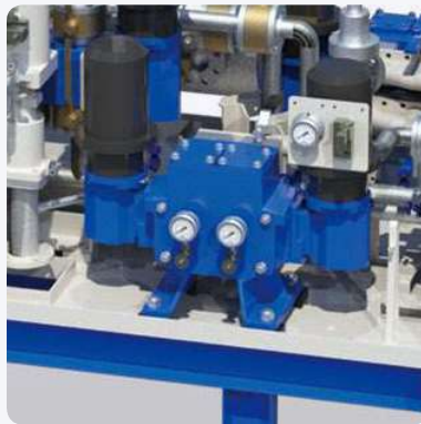
P-01 / 02, P-03 / 04 Supply Pumps, Circ. Pumps
